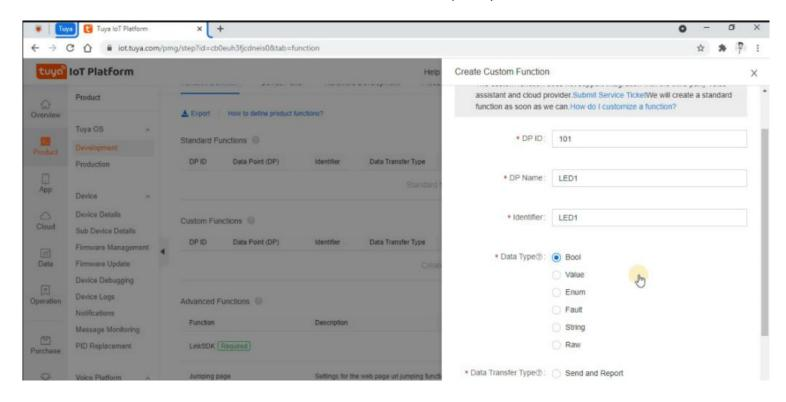
Similarly add the function for LED2, here LED2 has a variable brightness as you saw in the output, so it will take a variable data value from 0-100, so let's add this function in the custom function. This function has 102 as DP value.
