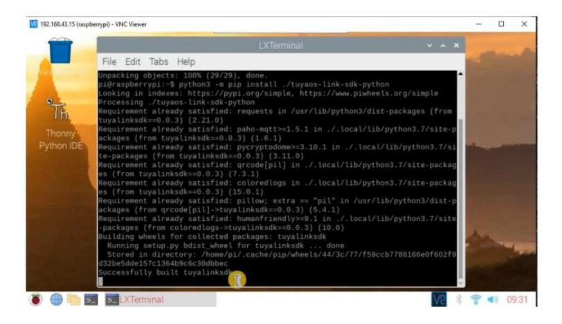
Now we have successfully installed the these thing now its time to run the code for which we have designed. But before this update the some parameter in the 'outlet.py' file which is present in the 'Tuya Link SDK python' folder, go and open that file and change the product, UUID and Authkey in this file.
