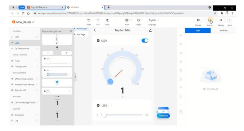
After that click on save then click on release button, this process take some time to apply the changes. At the end it will ask for the test or apply here click on test button to test the GUI, is it working or not?
